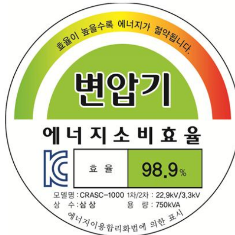
Figure 1. Korean Label for Distribution Transformers
