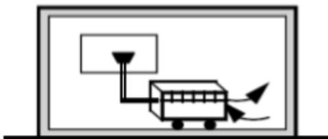
Double duct units are similar to single duct units but take the air to cool the condenser from the outside as well. Sometimes these are wall-mounted, with concentric ducts through a hole in a wall or via a flexible duct (mobile units). Double duct products units are tested using the same standards
